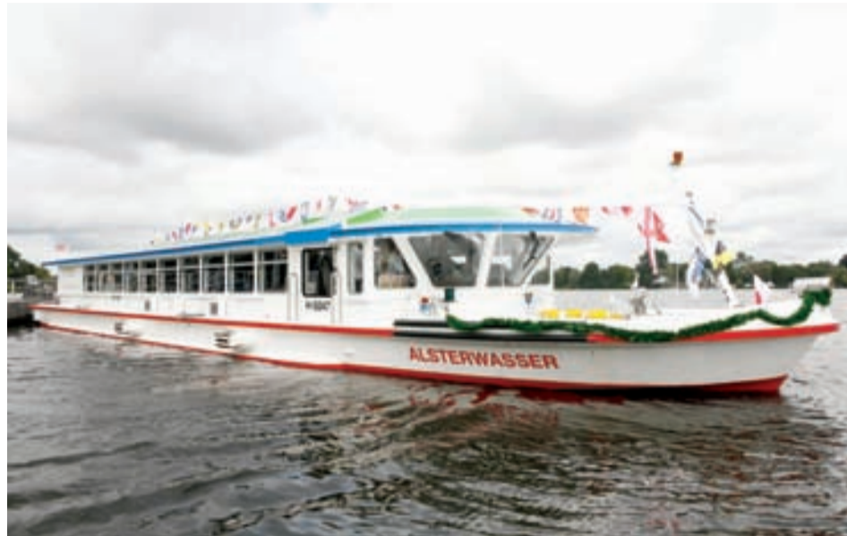
The Alster Wasser, powered with hydrogen fuel cells, is already operating on Hamburg’s Alster Lake – Photo: HOCHBAHN
